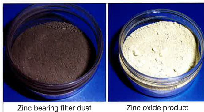
Fig. 6: Comparison input filter dust and zinc oxide product
